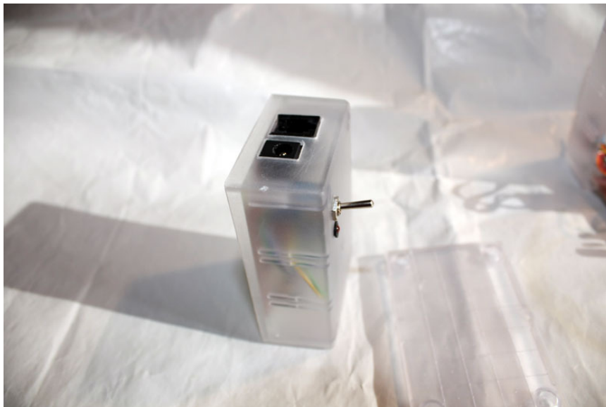
Assembled Module. Note where I placed the switch and power LED, away from transceiver.
