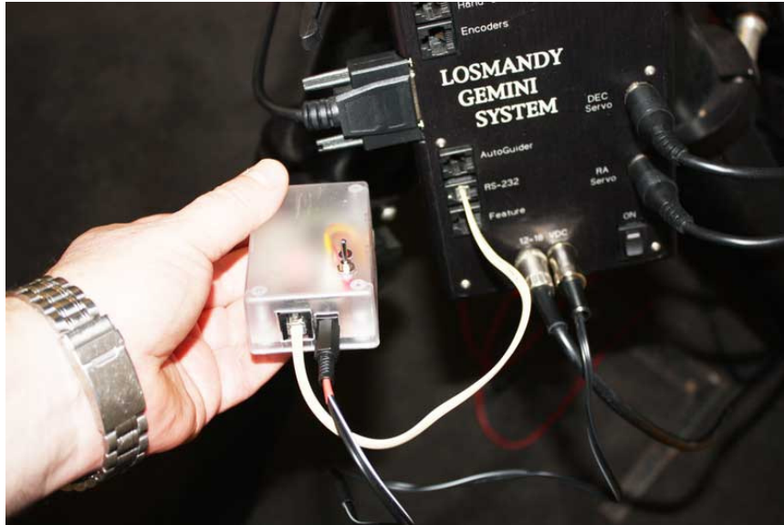
Shows power and RJ11 connections between components.
